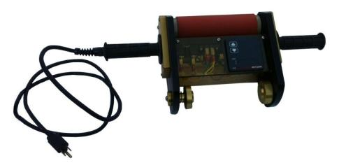
The I.F.P. system allows easy manipulation of the three basic principles of successful foil stamping; heat, pressure, and dwell time. Heat for both the printer and the hot plate may be precisely controlled between 100°-260° F. With this system the the foil can be adhered using the pressure that one average person may bring to bear on the foil and substrate. The dwell time is easily manipulated and can be extended to the point of tedium.
